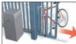
entrapment prevention system reverses gate on contact
