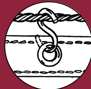
Cable & S-hook Installation
